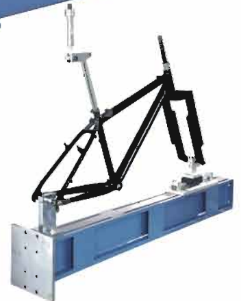
DBG008-E Frame with Steel Bar Fatigue Test
