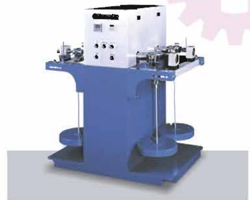
HT-2334 Bicycle Hub Abrasion Tester
