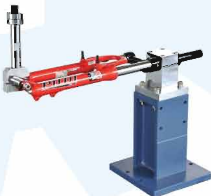
DBG001-B Front Fork Fatigue Test (Horizontal Test)
