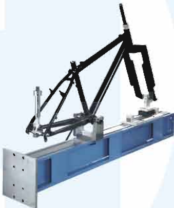
DBG008-C Rear Ends / Dropouts Fatigue Test
