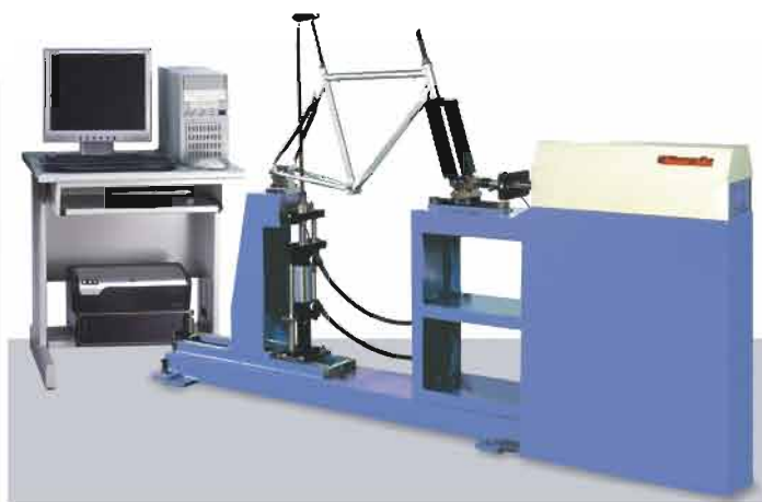
HT-2707PC Bicycle Frame Horizontal & Vertical Dynamic Fatigue Tester ( Pneumatic Type )
