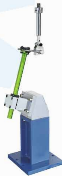
DBG007-F Seat Post Fatigue Test ( Single Force )
